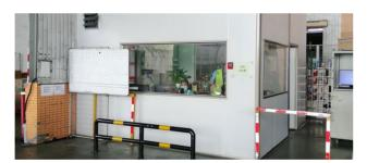
Soundproof operator booth installed in noise zones
